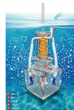
Nanobubbles are generated in the pure water tank and sterilized by crushing the nanobubbles
