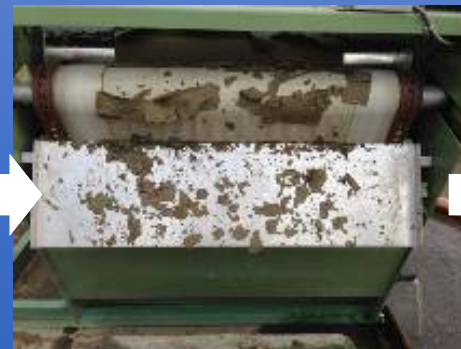
Sludge after press drying
