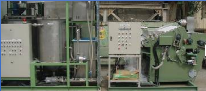
Condensation mixing equipment
